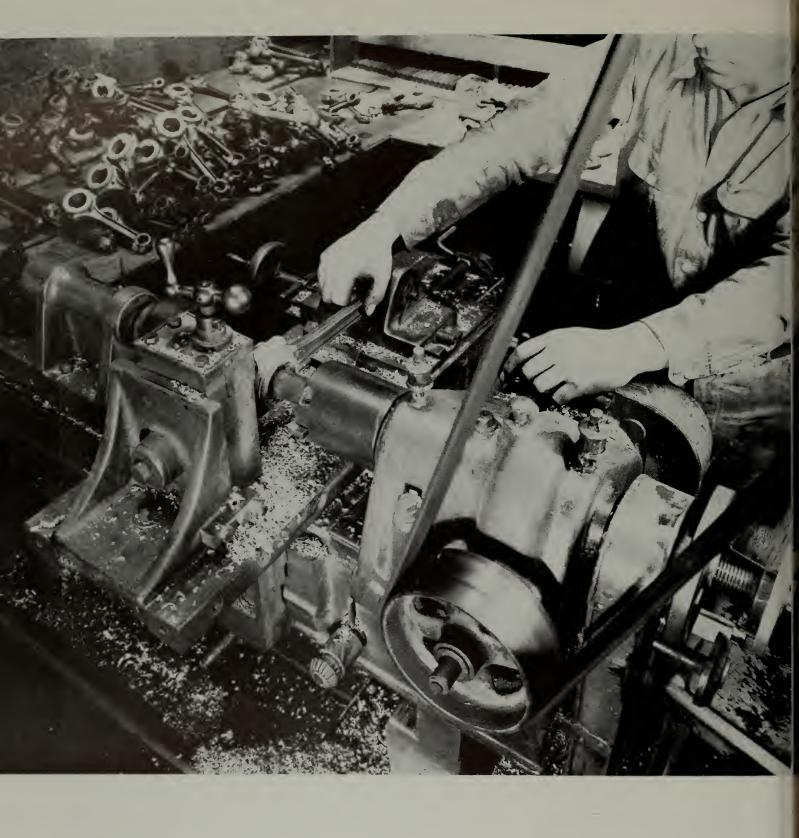
The rod is now placed in a lathe and the babbitt is bored, faced and chamfered. The latter two operations finishes the bearing to standard width.
